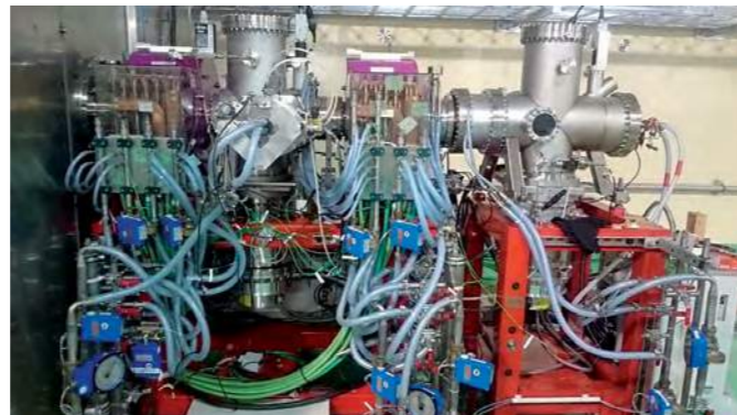
Low Energy Beam Transfer installed in Rokkasho, Japan
