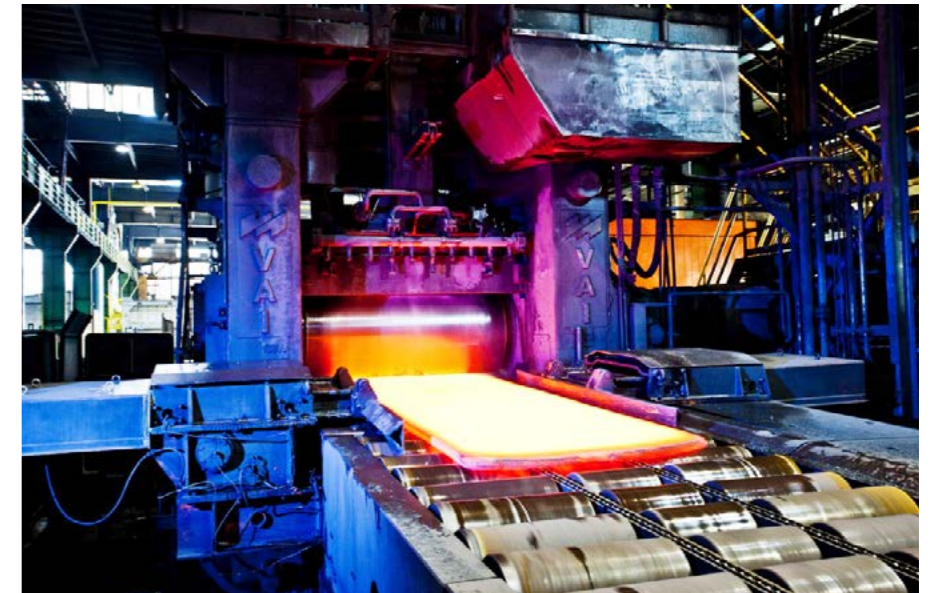
Rolling the EUROFER97 plates at Bohler Bleche
