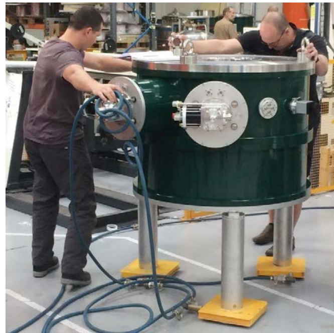
The magnet which will be joined to the gyrotron prototype and tested at Swiss Plasma Center
