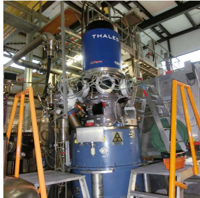
The 1 MW gyrotron prototype manufactured in Europe by French company TED on behalf of F4E
