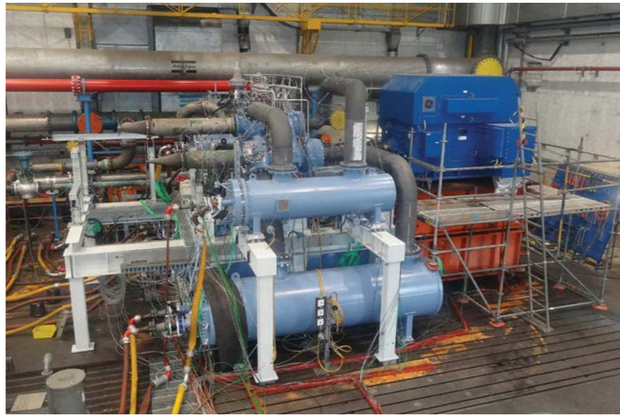
Nitrogen compressor of the ITER LN2 plant successfully tested at Atlas Copco
