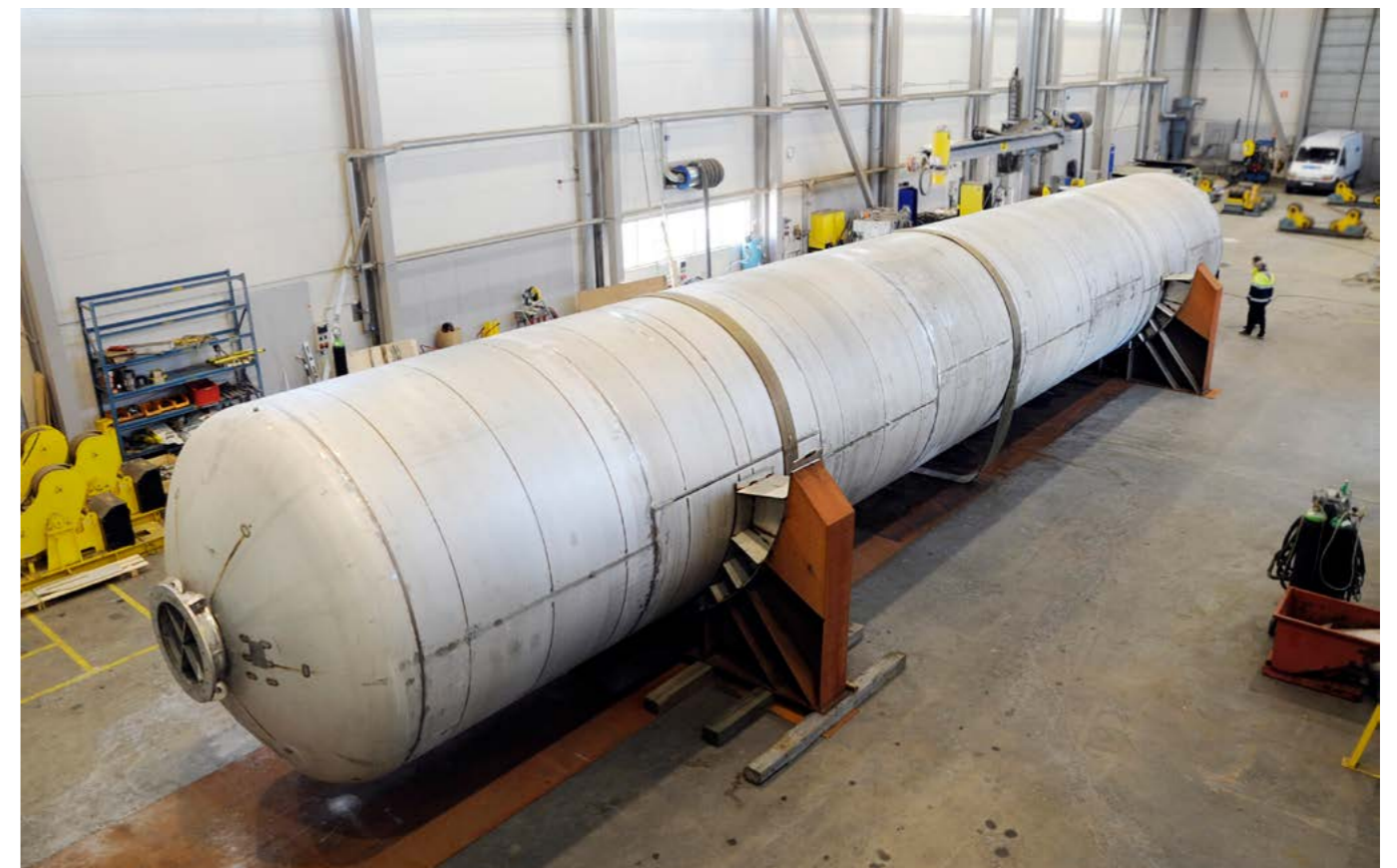
The liquid helium inner-tank, designed and manufactured by CryoAB, part of the contract signed between Air Liquide Global and EC Solutions and F4E, February 2016
