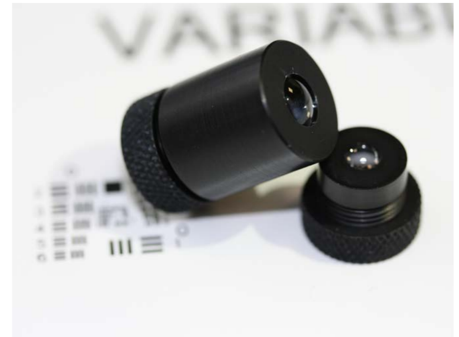
Mock-up of the optical subsystem part of the FURHIS project (Fusion for Energy Radiation Hard Imaging System) signed between F4E and OTL
