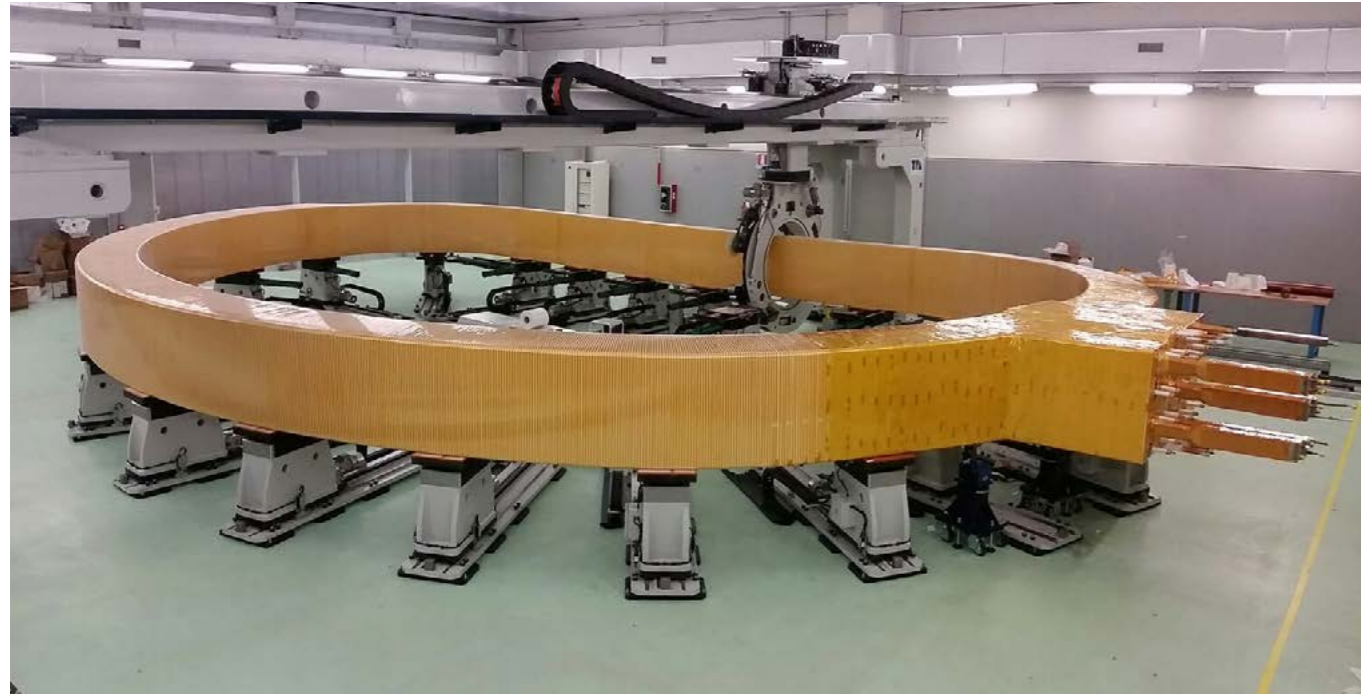
Performing ground insulation on the winding pack prior to impregnation, ASG, La Spezia, Italy
