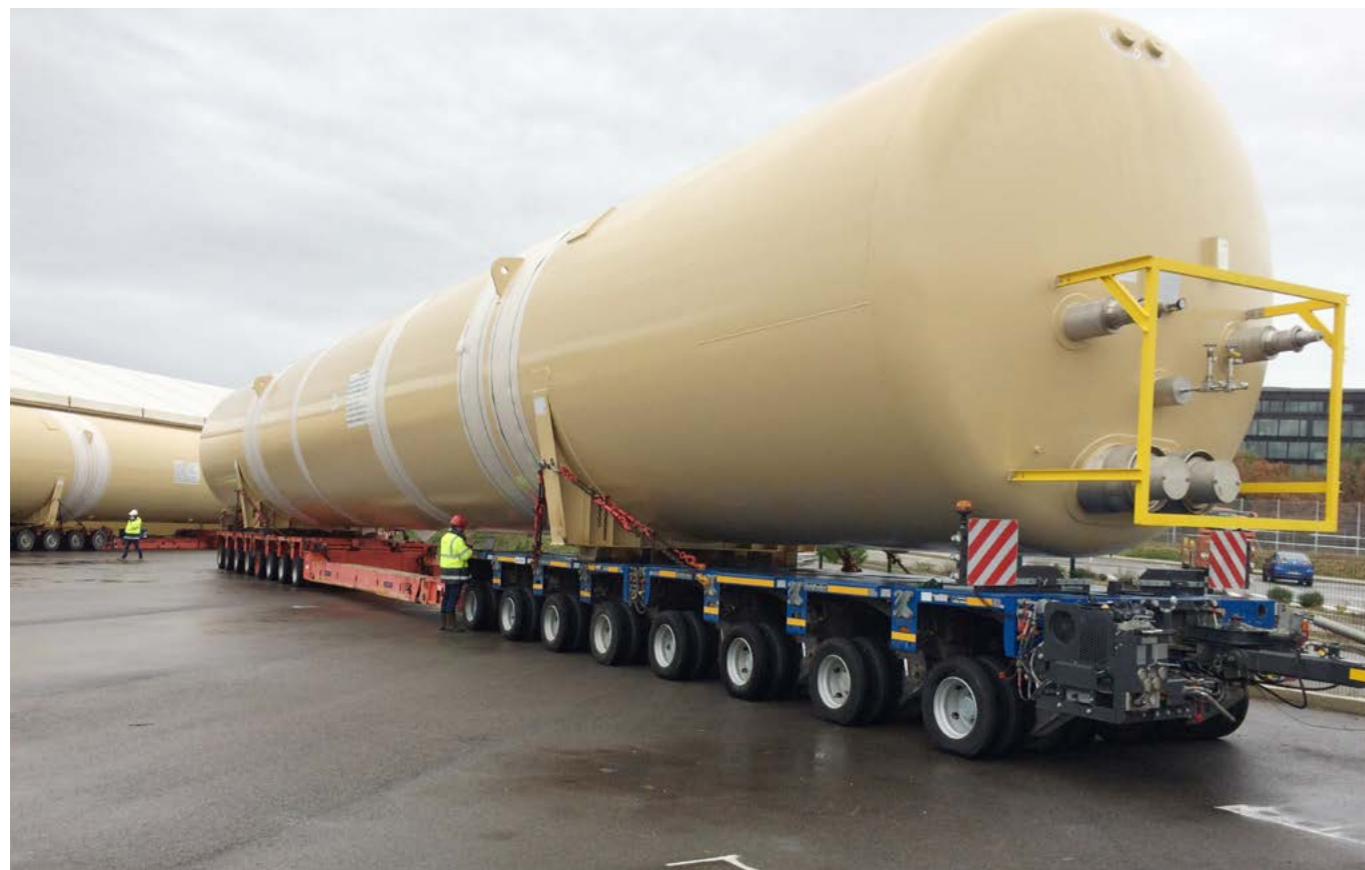
One of the two quench tanks stored at the ITER worksite. Manufactured by Air Liquide and their subcontractor Chart Ferro, it is 35 m long and has a diameter of 4.5 m. It weighs approximately 160 T.
