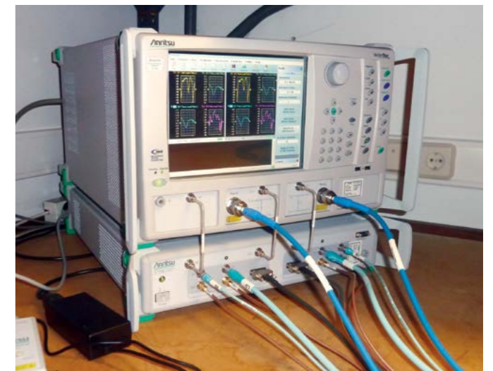
The Vector Network Analyser measuring device used to qualify ITER diagnostic components
