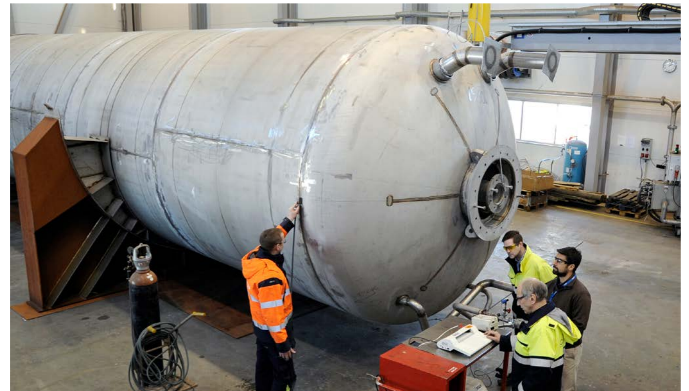
CryoAB technicians carrying out the liquid helium leak test on the inner-tank. It took almost half a day to inspect roughly 500 m of linear welds. February 2016
