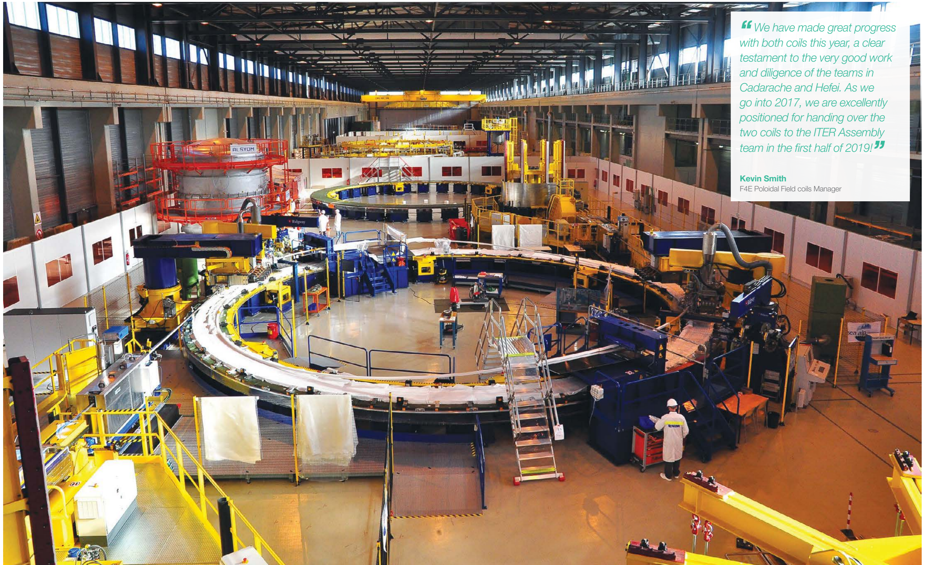
Winding tooling at the Poloidal Field coils Facility where cleaning, sandblasting, bending, insulation and wrapping of the conductor will be performed, Cadarache, December 2016 ©ITER IO
