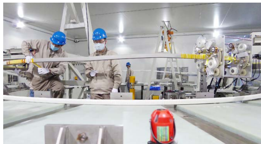
Top image: Team of technicians checking the manufacturing of the insulated dummy conductor, ITER Poloidal Field coils Facility, Cadarache, November 2016
