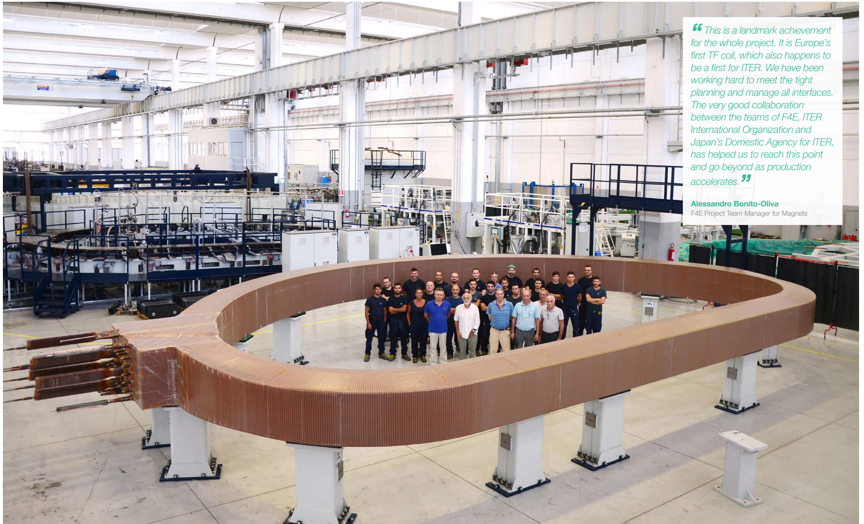
First impregnated winding pack, the core of an ITER Toroidal Field coil, ASG Facility, La Spezia, Italy
