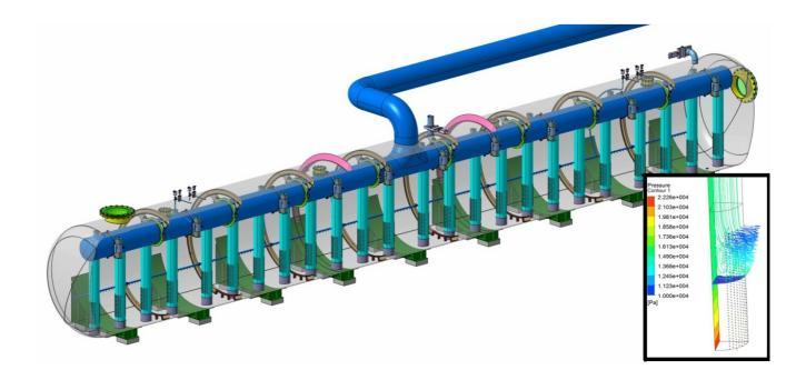
**Figure 1.0** Vacuum Vessel Pressure Suppression System (inset – sparger)
