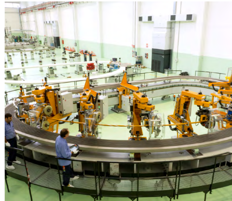
Wrapping and insulation of conductor for the ITER Toroidal Field coils, ASG, November 2015
