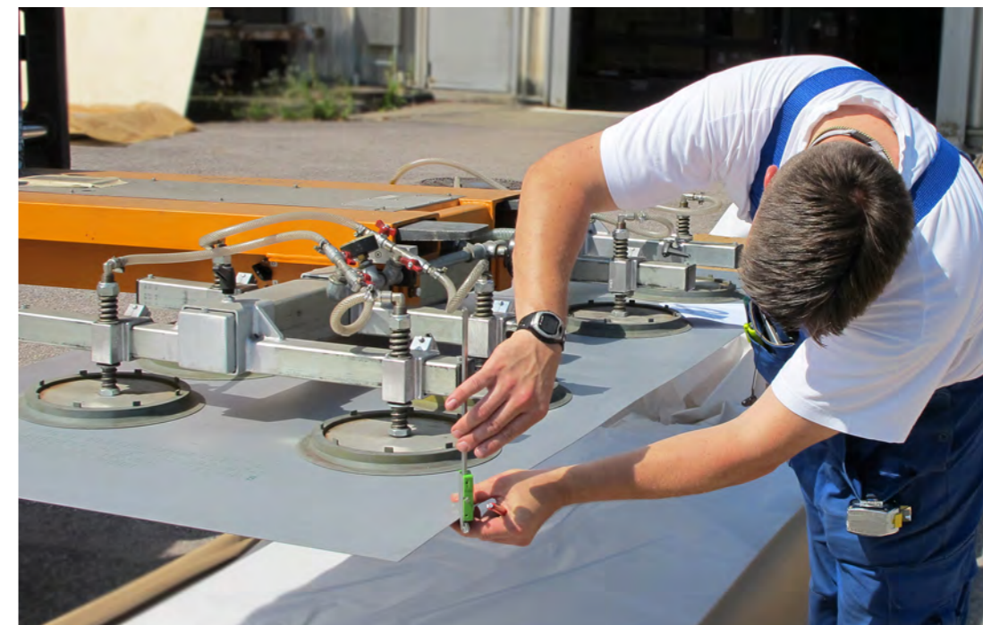
Technical staff measuring the thickness of the EUROFER plates
