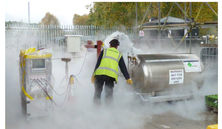
Heatric technical staff carrying out the liquid nitrogen test.
