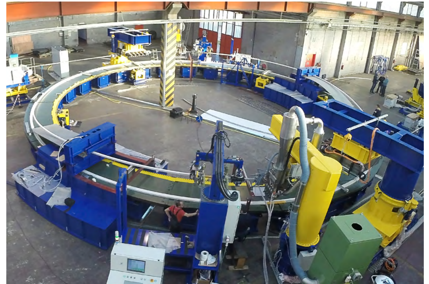
The Poloidal Field coils winding tooling table, SEA ALP workshop, Turin (Italy)
