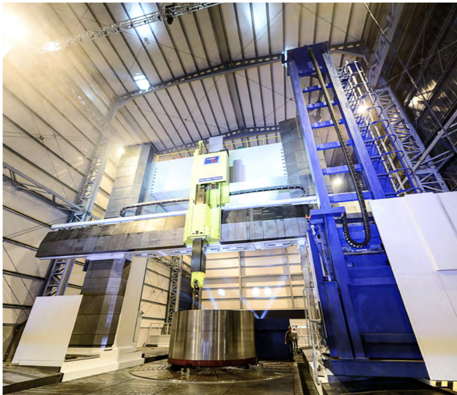
The milling machine inaugurated at the Water Tosto facility for the manufacturing of the ITER vacuum vessel sectors (image courtesy of Waldrich Coburg)
