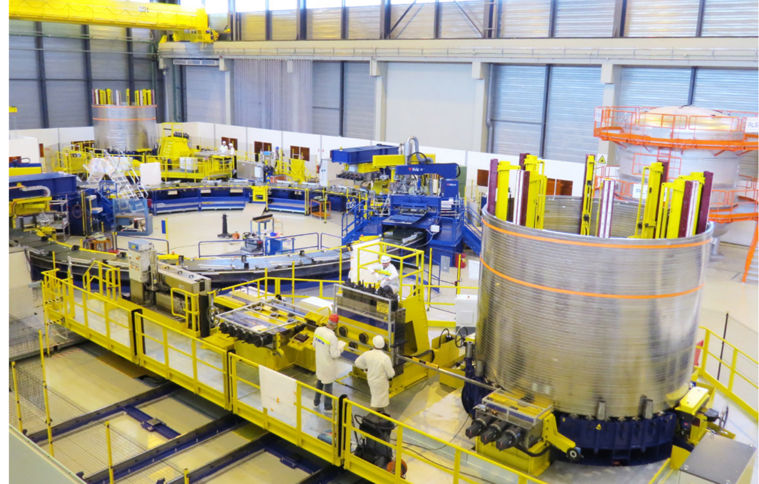
CNIM technicians supervising the manufacturing of the European Poloidal Field coils in F4E's facility, Cadarache
