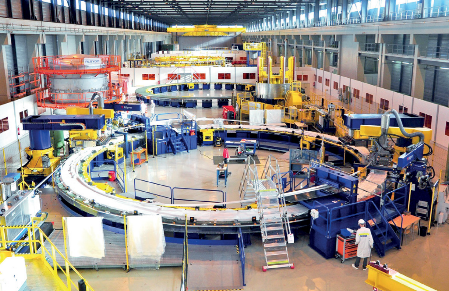
European contractors have completed winding a full-size dummy double pancake for the fifth Poloidal Field coil, Cadarache © ITER IO
