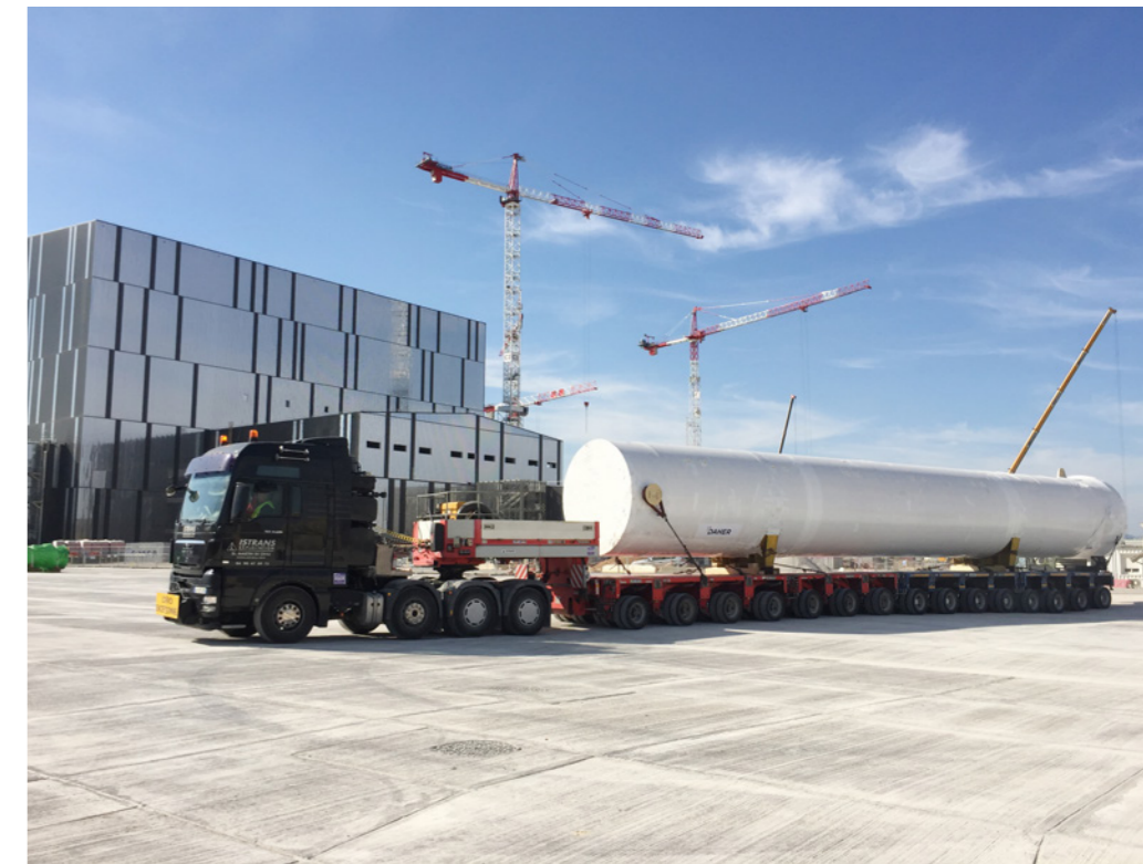
The GN2 buffer tank, part of ITER's Cryogenic system, has been delivered on-site, Cadarache, October 2017
