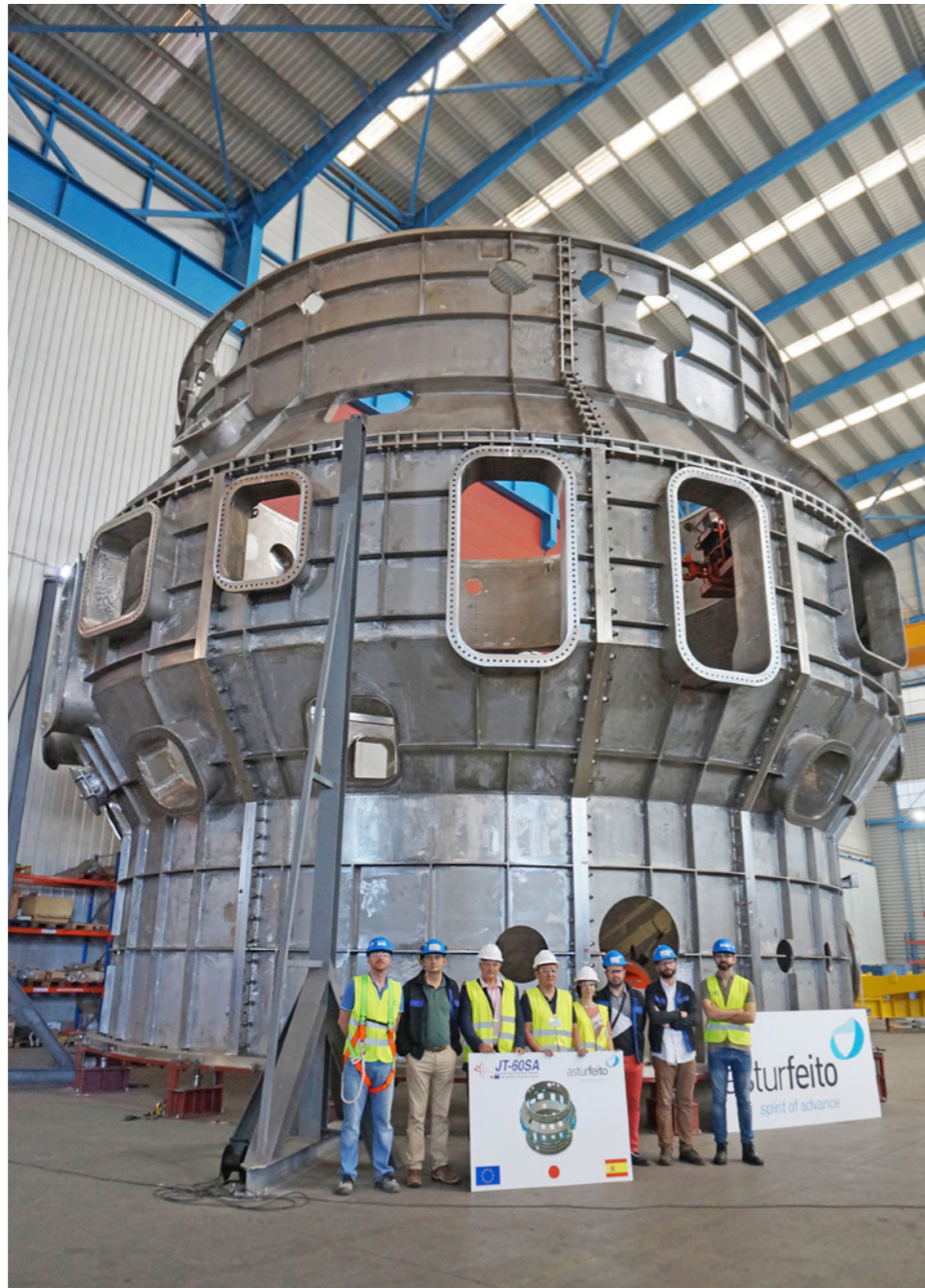
The F4E/CIEMAT/Asturfeito S.A. team in front of the JT-60SA cryostat vessel body.
