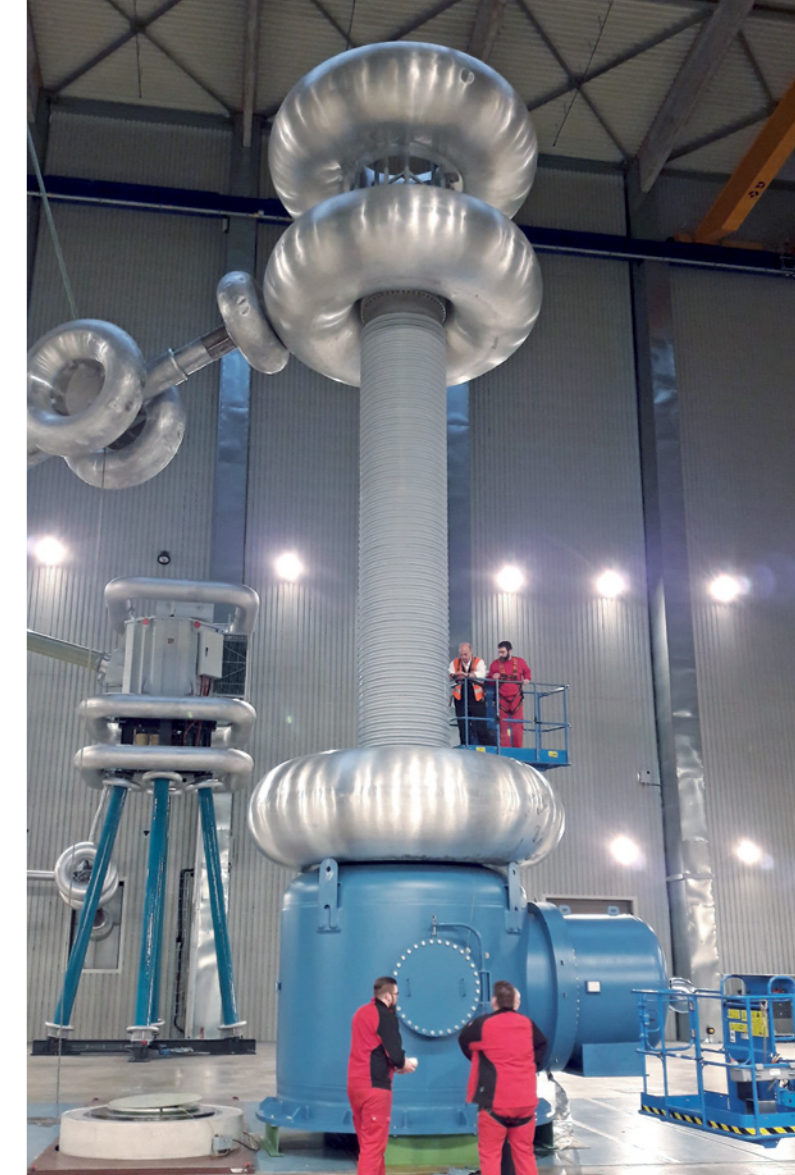
High Voltage Bushing during electrical tests, HSP GmbH high voltage facility, Germany. © SIEMENS
