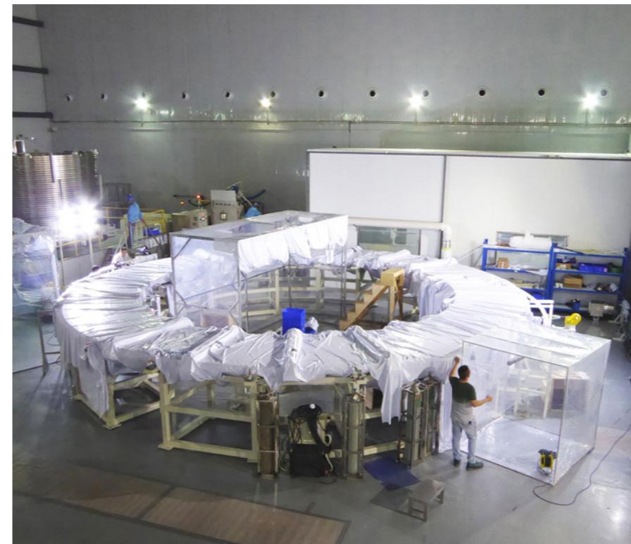
Working on the terminations of one Double Pancake of Poloidal Field coil 6, ASIPP, China
