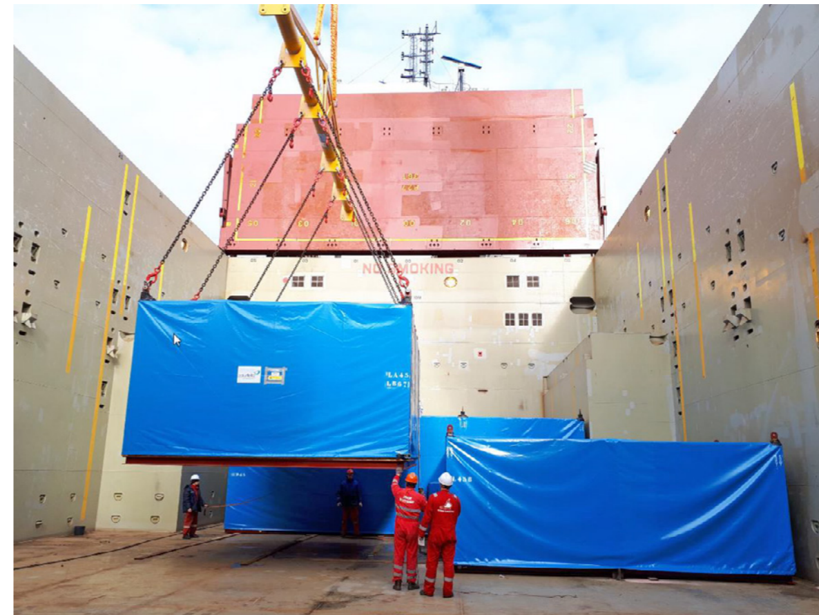
36 packages and the two lifting devices weighing a total of 322 t have been loaded on the ship © DAHER
