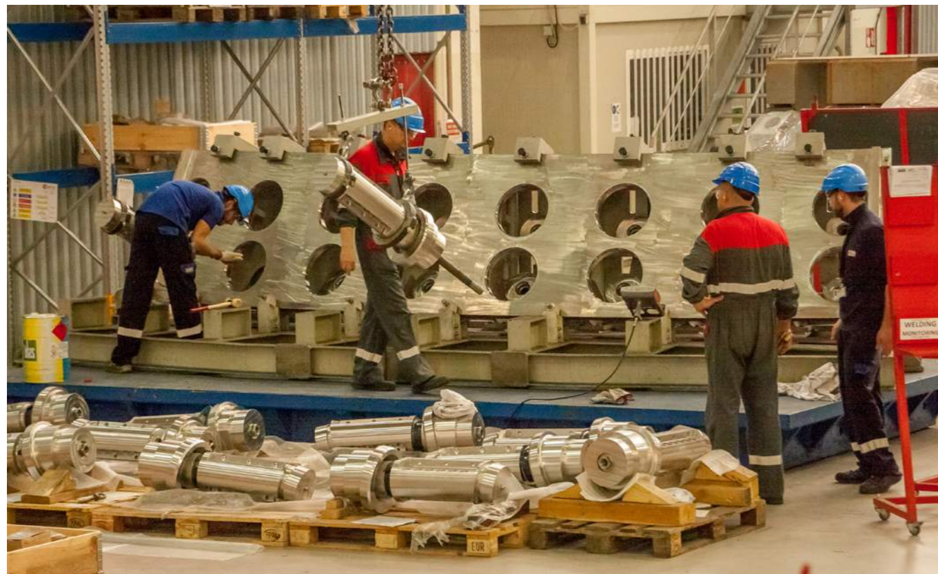
Workers at Mangiarotti S.p.A installing the forgings (in the foreground) in one of the plates (in the background).
