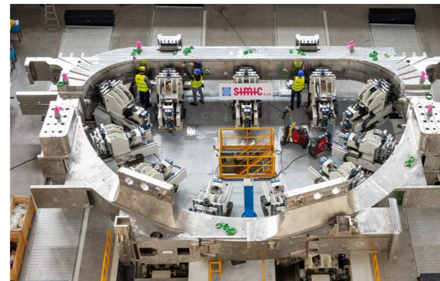
Europe's winding pack inserted into its case coil, SIMIC, Port of Marghera, Italy. It is the first time that this operation is performed in the history of the ITER project © SIMIC
