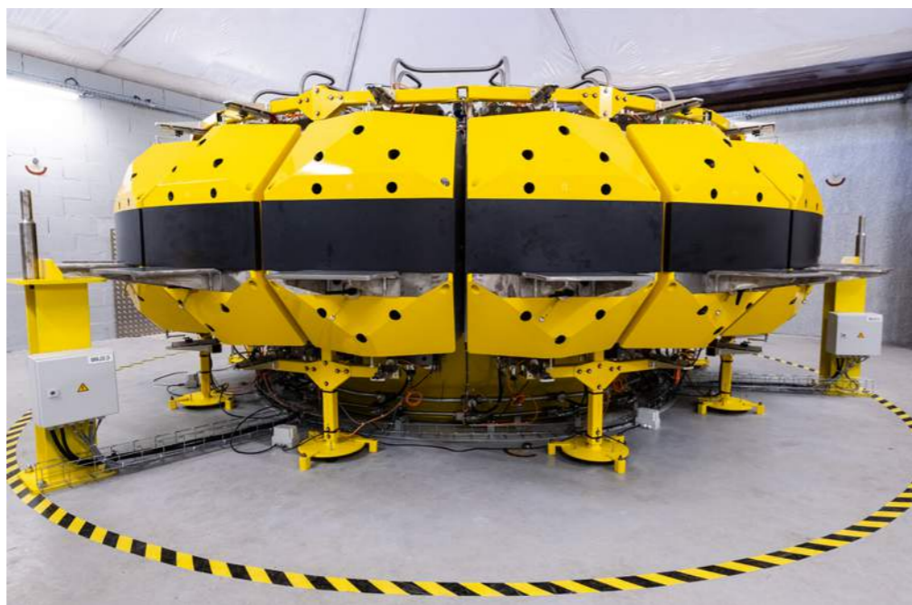
The tooling which will be releasing a force of 36 000 t to test the quality of the ITER Pre-Compression Rings, CNIM, La Seyne-sur-Mer, France.
