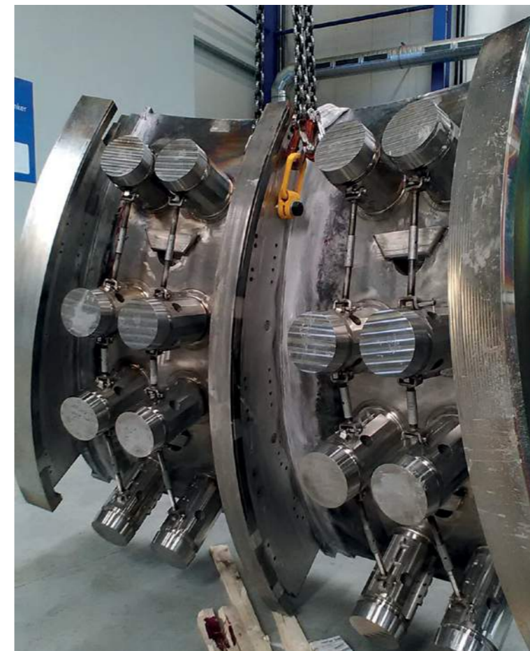
The top sub-assembly for the second segment for sector 4 manufactured by Walter Tosto for the Vacuum Vessel ready for electron-beam welding at Pro-beam.
