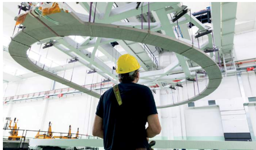
Technician lifting a Double Pancake, ASG Superconductors, La Spezia (Italy) © Andrea Botto
