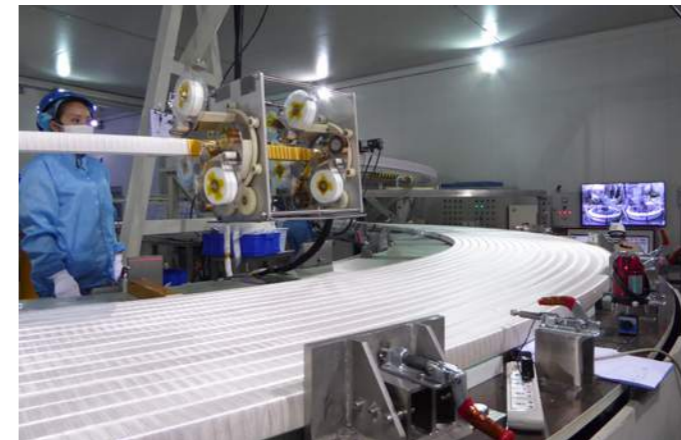
Wrapping and insulating with Kapton and fiber and glass tapes the conductor of the sixth Poloidal Field coil
