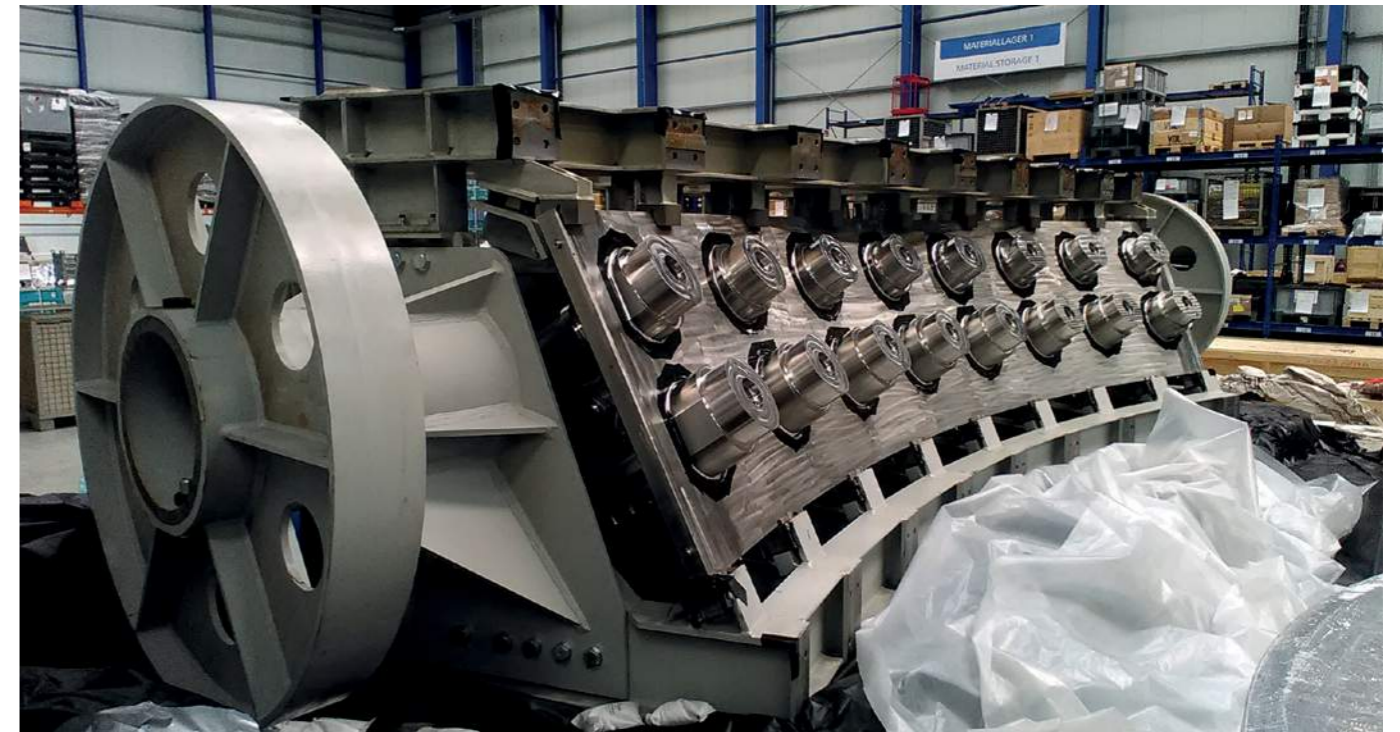
The triangular support subassembly for the fourth segment for sector 5, manufactured by Mangiarotti and electron-beam welded at Pro-beam.
