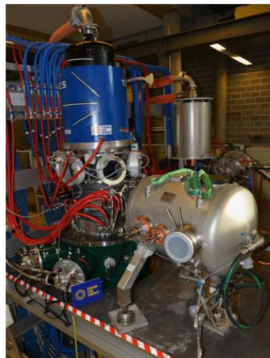
Tests on-going in Falcon facility, Swiss Plasma Centre, where the European gyrotron is located
