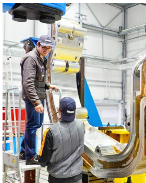
European real-size prototype of ITER Divertor Cassette manufactured by CNIM – SIMIC © CNIM
