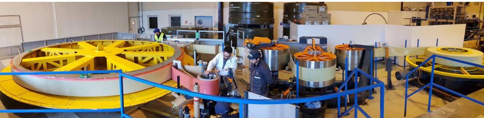
Technicians checking the tooling, performance of material and the method to produce the ITER Pre-Compression Rings © CNIM
