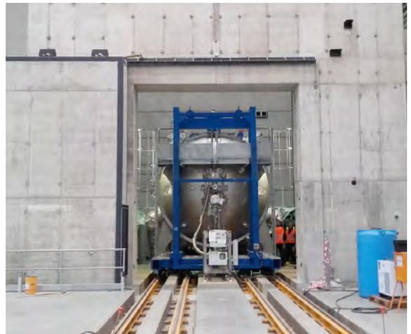
The SPIDER vacuum vessel inside the bio-shielding
