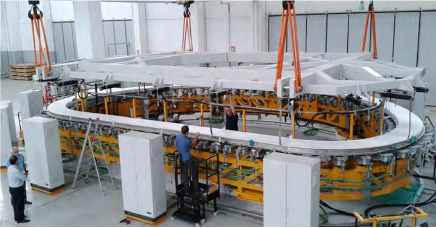
Assembly of a series DP on the VPI mould, ready to be impregnated in ASG, La Spezia (Courtesy of ASG)
