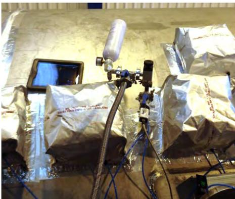
Helium leak test of 100 m<sup>3</sup> tank
