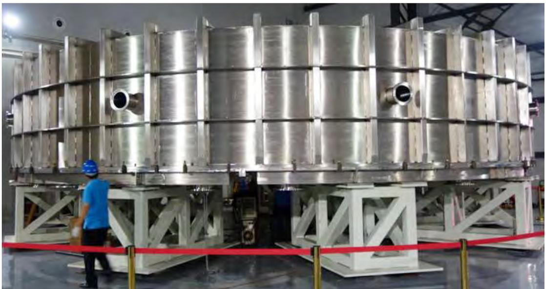
Some of the developments carried out at the ASIPP facility in Hefei, China and its suppliers: View of the PF6 DP Vacuum Chamber during commissioning at ASIPP
