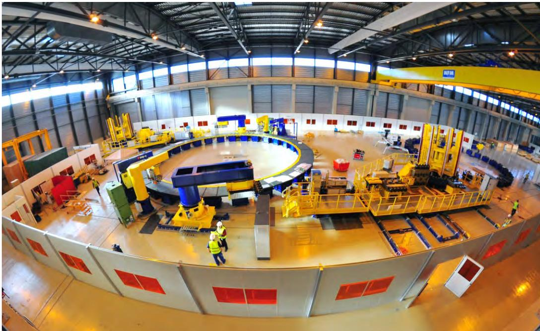
PF 2-5 Winding Machine installation in the PF Building at the Cadarache site
