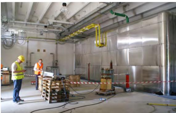
*The SPIDER High Voltage Deck during tests*
