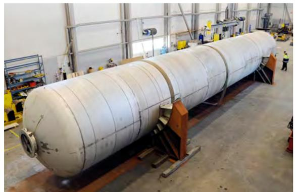
*LHe tank inner vessel helium leak test*
