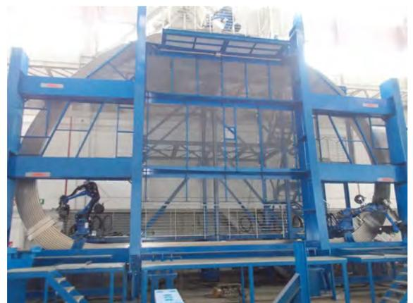
The three big sectors of the Radial Plate are being welded in the welding frame at the SIMIC site (Courtesy of SIMIC)
