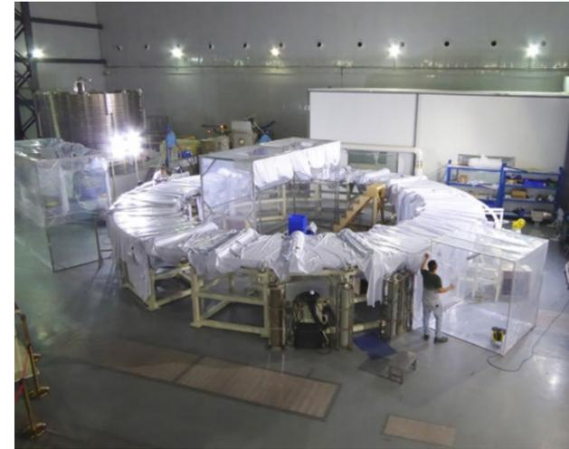
Working on the terminations of one Double Pancake of Poloidal Field coil 6, ASIPP, China
