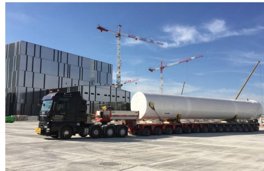
The GN2 buffer tank, part of ITER's Cryogenic system, has been delivered on-site, Cadarache, October 2017
