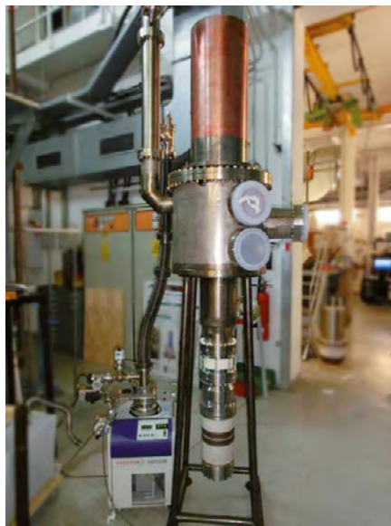
Fabrication and testing is currently being carried out on the short-pulse gyrotron.
