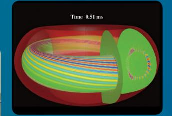
This simulation of the spatial distribution of a particular type of instability in an ITER steady-state plasma shows that it would not degrade the confinement of alpha particles
