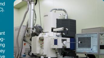
Field emission scanning electron microscope
